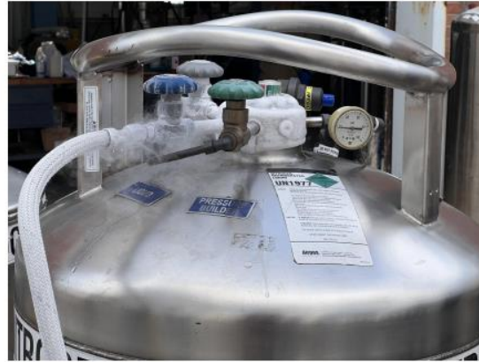
Liquid Nitrogen used for condensing Argon gas after purification.
