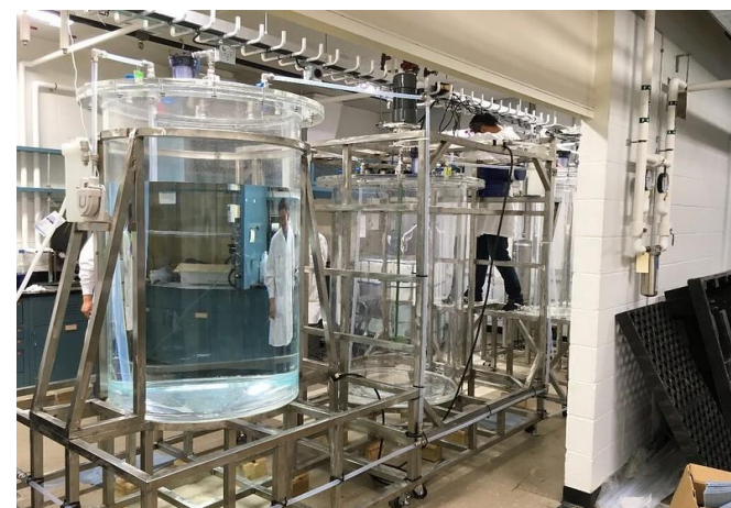
1000 L Sequential-Mixing Reactor System in Liquid Scintillator Production Facility (LSPF) at BNL.
