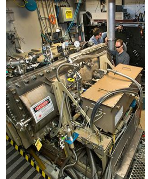
BNL's ATF is the only laser facility in the world operating with a picosecond-and terawatt-class CO2 laser in the Chirped Pulse Amplification (CPA) regime.
