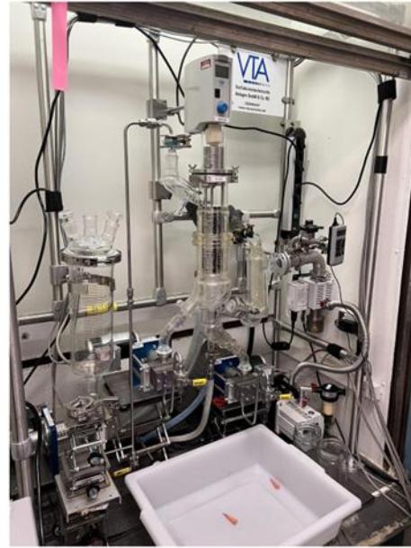
Thin-film Vacuum distillation system for purification for liquid scintillator.
