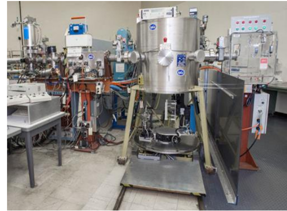
Single Event Upset Test Facility at BNL's Tandem van de Graaff accelerator.
