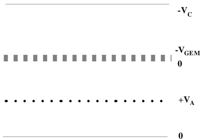
Fig. 4: Test assembly with the GEM multiplier mounted within a standard MWPC (drawing not to scale).
