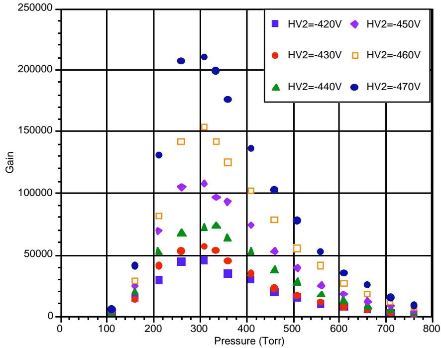
Figure 3. Measured gain in He + 6% Isobutane as function of the gas pressure for various potentials applied on the micro-grid.
