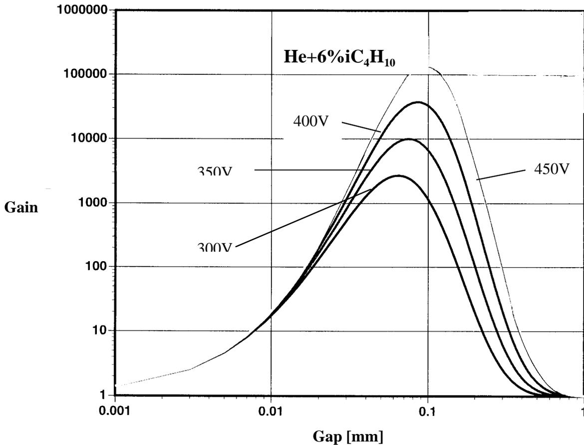
Figure 2. Calculated gas gain in He + 6% Isobutane as a function of the amplification gap for various potentials applied on the microgrid.
