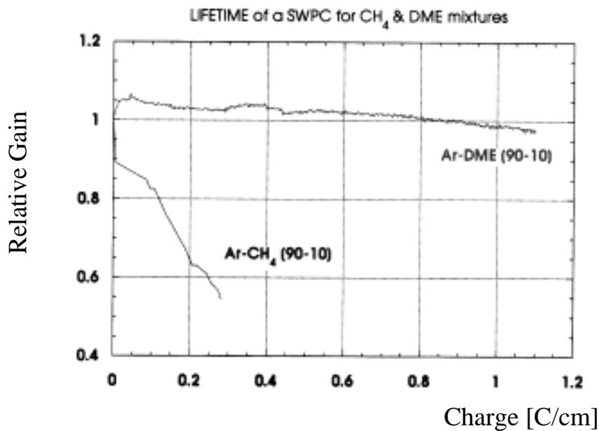
Figure 11 Comparison of the response of a clean single wire proportional counter irradiated in Ar-DME and Ar-CH<sub>4</sub>.
