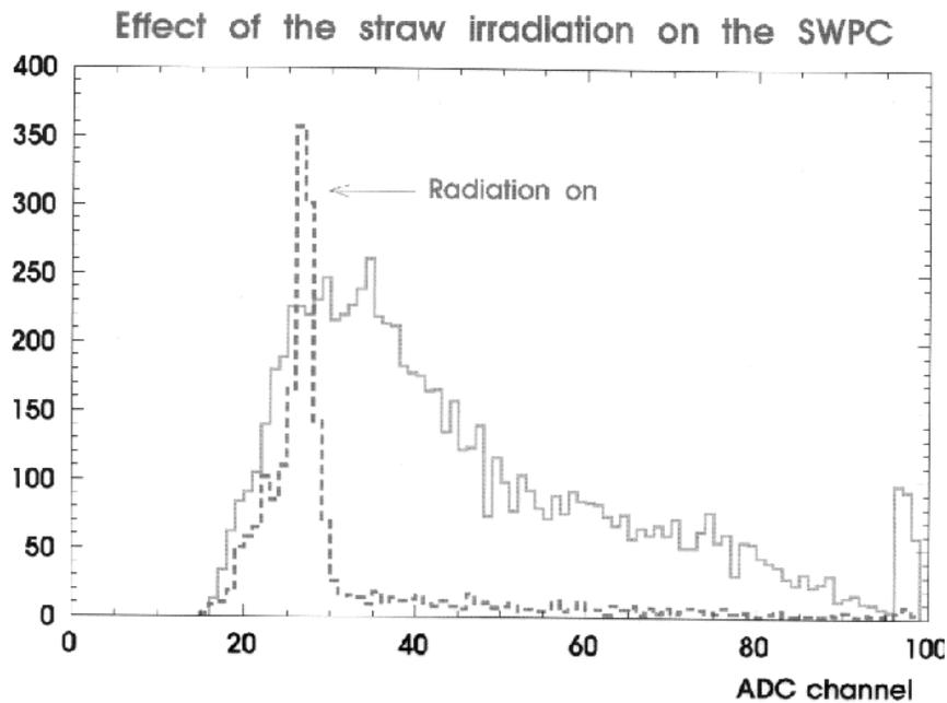
Figure 13 Pulse height measured in a single wire proportional counter (3 cm drift distance), which is gently irradiated but connected downstream a small diameter straw tube in Xe-CF<sub>4</sub>-CO<sub>2</sub> (50-30-20). When the straw tube is strongly irradiated the large energy pulses (continuous line) are suppressed due to the effect of electronegative species created in the avalanche.
