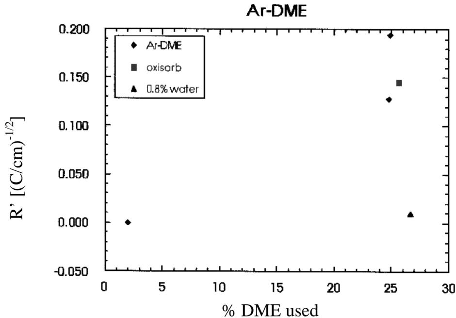
Figure 12 Aging rate for several tests carried put with Ar-DME (90-10) expressed as  $R'$  as function of the use of the DME cylinder. The triangle point corresponds to the rate of aging measured when 0.8% of water is added to the gas mixture.
