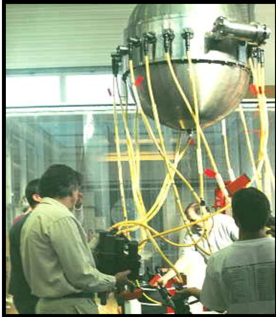
Fig. 20a Antares junction box with penetrators and underwater-mateable connectors
