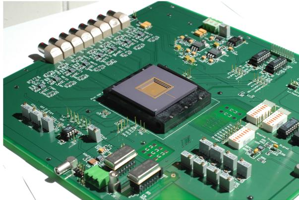
Figure 7: Photo of the large area ASIC mounted on the control motherboard.
